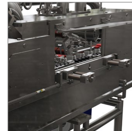
Central adjusting of the side belts
