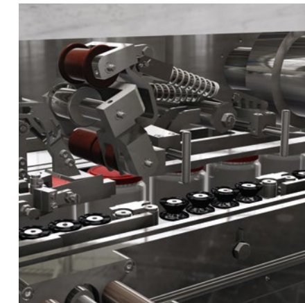
Cap transfer. Press-on device and cap strap in their 50-year-approved stainless standard
